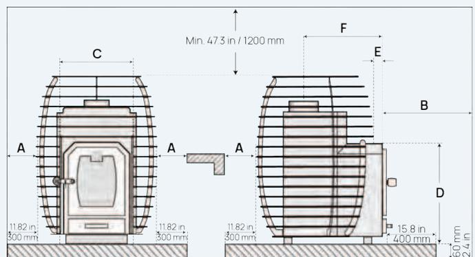
\* In case the HIVE Wood heater is installed near combustible material and necessary safety distance cannot be guaranteed, use a heat reflector to reduce the safety distance by half.
