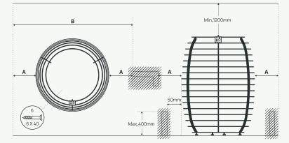
\* In case the heater is installed near combustible material and necessary safety distance cannot be guaranteed, use a heat reflector to reduce the safety distance by half.
